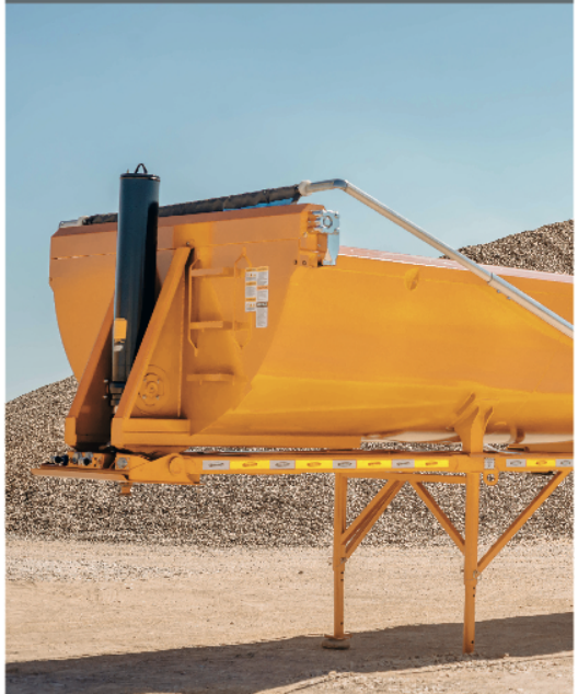
Front to back oscillating fifth wheel
