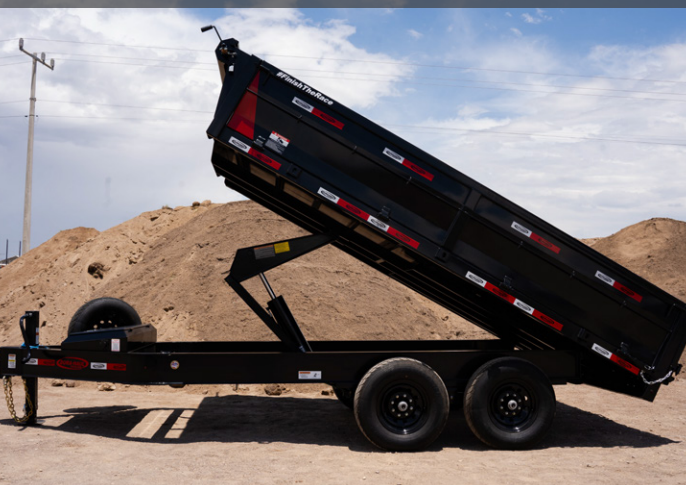
Heavy duty hydraulic scissor 45° lift angle
