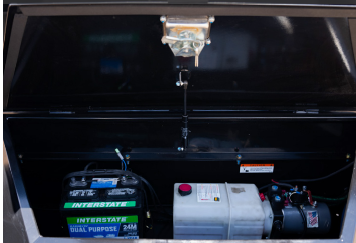
Lockable tool & equipment box, charger, pump, battery & remote control
