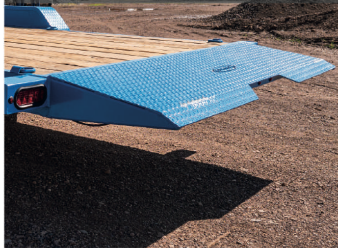
3/16 gauge diamond plate rear ramp
