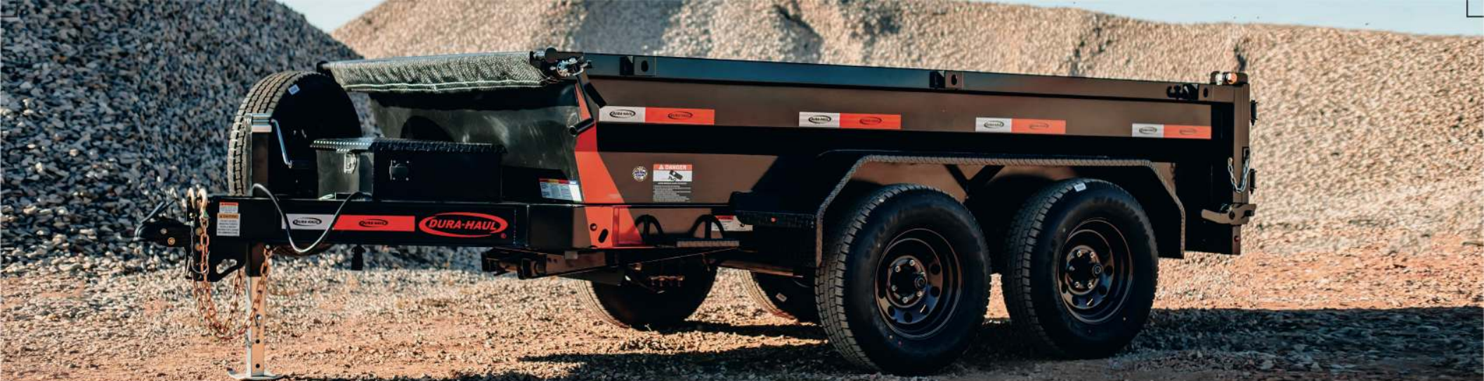
Heavy duty hydraulic scissor lift, 45° lift angle
